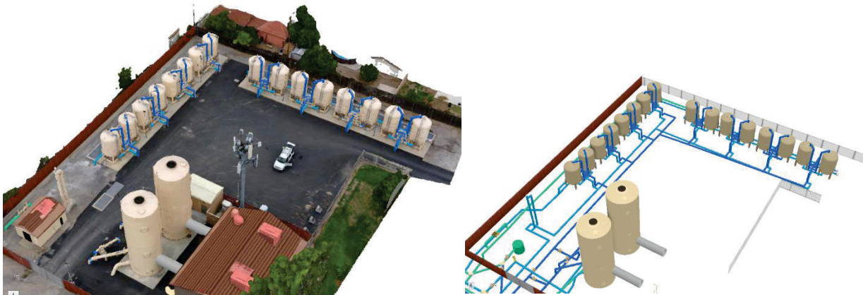
Figure 9 – Left side - Sample Drone Model overlaid with UN Data, Right side – UN data in 3D View , refined per Drone model.
